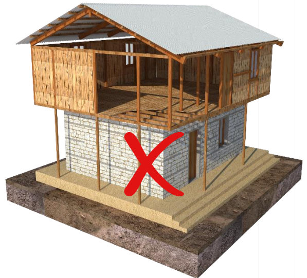
The wall line is not on the wall line of lower storey
