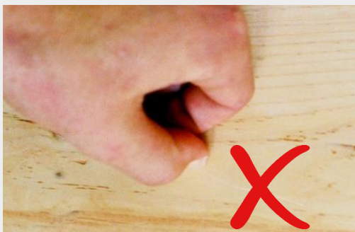
When pressed by tip of nail leave a mark (Soft wood)
