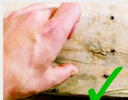
When pressed by tip of nail doesn't leave a mark (Hard wood)
