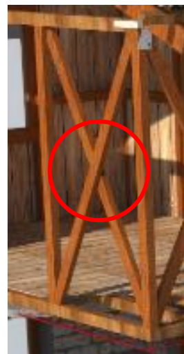
It should be fixed by nail Nail: length 75mm x 4
