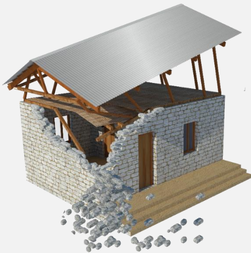
Failure of ground floor
